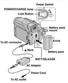
This camcorder's 2-way power supply system lets you choose the most appropriate source of power. Do not use provided power supply units with other equipment.
